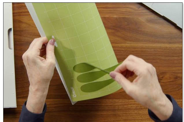
Curl the mat, and the front edge of the cut will pop up
